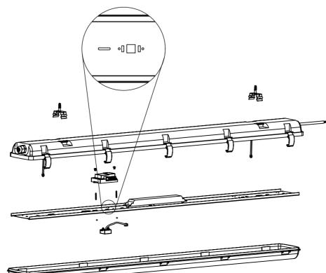
Wire with included instructions (VTS-SENSORKIT). Wire fixture in accordance with national, state, local and electrical codes.
