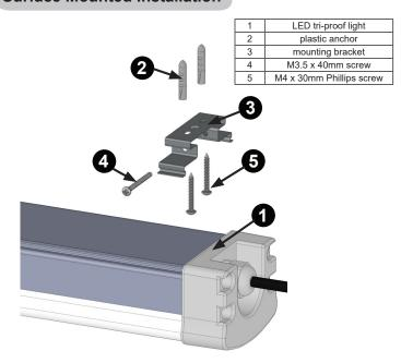
Drill two pairs 15/64" holes on the ceiling or wall. These should be spaced as indicated in provided application table for length and 1" to 1 1/16" apart to accommodate bracket.
