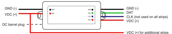
Note: Wire colors may vary by strip. Make sure to connect the wiring correctly to avoid malfunction or potential damage to components. Controller also features a 5.5 mm/2.1 mm DC barrel plug that can be used to connect to input power.
