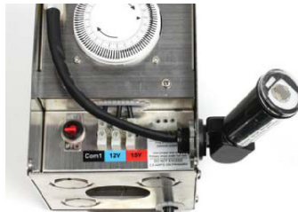
3. Insert the wire and connector of photocell through hole in side of transformer. Place nut around wire and screw onto photocell, holding unit in position.
