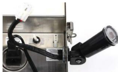
3. Insert the wire and connector of photocell through hole in side of transformer. Place nut around wire and screw onto photocell, holding unit in position.
