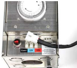
3. Insert the wire and connector of photocell through hole in side of transformer. Place nut around wire and screw onto photocell, holding unit in position.
