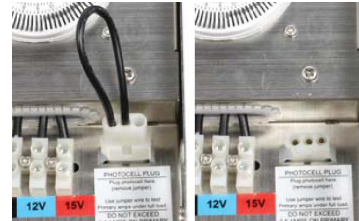
2. Unplug photocell plug from transformer.
