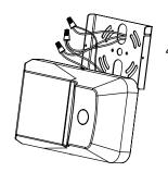
I. Use slots to temporarily hang light on mounting bracket to J-box. Make wire connections to main supply. Push connected wires through bracket into J-box.
