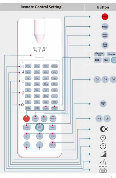
As the control angle of the Infrared Remote Control is fixed (15°), if sensors are installed too close to each other, settings of both sensors will be configured. Please refer to the below chart for the distance of the installation of the sensor:
