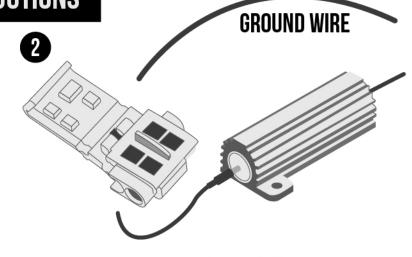
Locate your turn signal socket and identify your turn/brake wire and your ground wire using a voltmeter. With the vehicle off, insert ground wire into the through (run) location on the terminal splice tap. **DO NOT CUT YOUR VEHICLE'S WIRE.**
