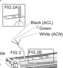
Cable to Junction Box Route the existing 30-inch cable to junction box near the fixture, making sure cable and connection are secure. Use the notch at end of the access plate to hold cable in proper position. (FIG 2B)
