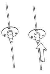
DRILL 6 ANCHOR HOLES AND INSTALL FLANGE
