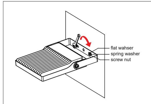
4. Fasten the nuts on the bolts to tighten the mounting bracket to the wall.(Fig 4)
