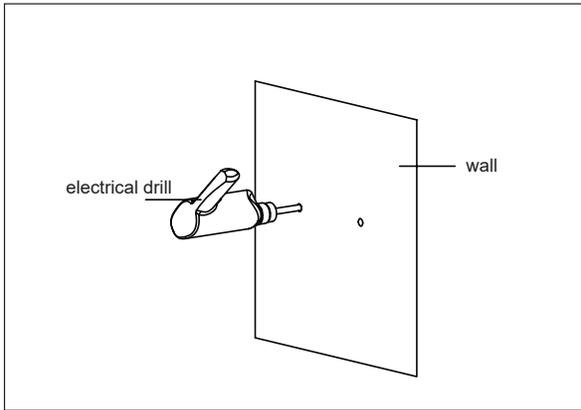
1. Use the mounting bracket to mark out bolt holes on the wall and then drill holes.(Fig 1)
