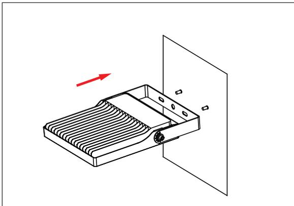
3. Place the mounting bracket over the bolts and push it flush with the wall.(Fig 3)
