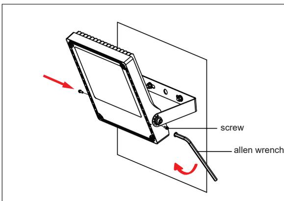
5. Rotate the light to the desired angle and tighten screws with an allen driver. (Fig 5)
