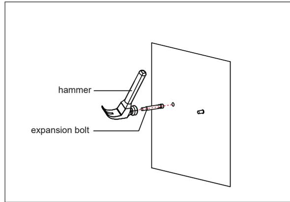
2. Drive the bolts into the holes with the threading facing outward.(Fig 2)
