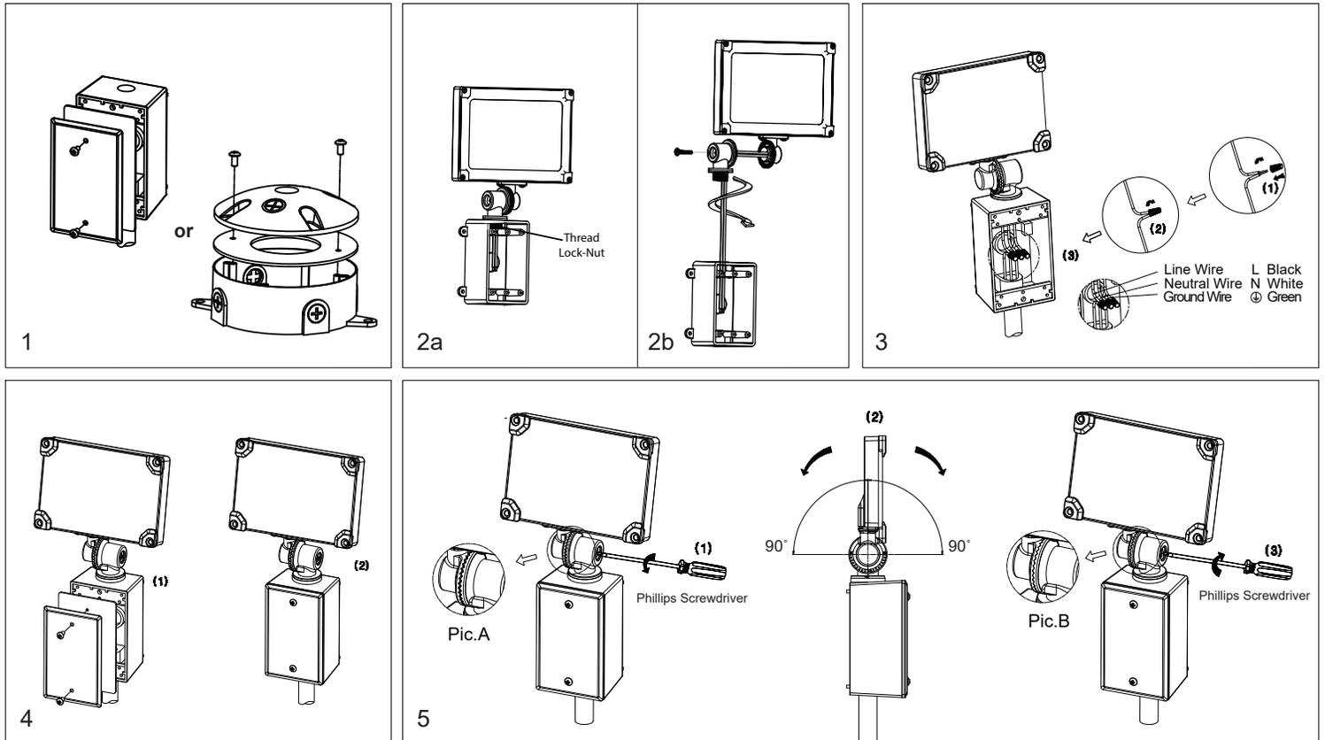
1. Use a screwdriver to remove junction box cover.
