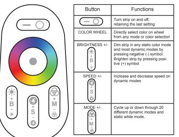
RF remote controller has a signal range up to 65ft (20m) and requires 2 x AAA batteries (not included).
