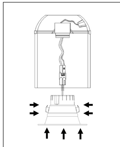
Note: 4-inch model (DL4D) shown. 5- and 6-inch model (DL56D) installs similarly, but utilizes a different style clip to hold the light in place.
