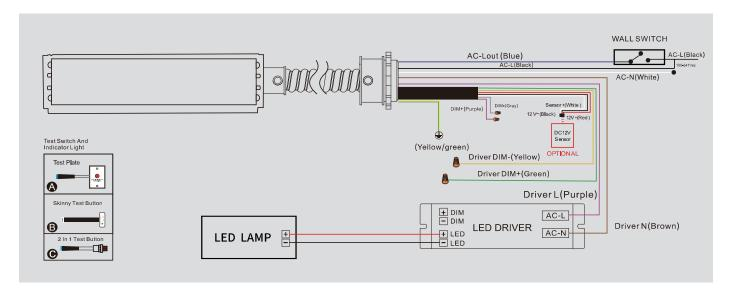
Emergency Driver can be used with either a switched or unswitched or emergency only fixture. If a switched fixture is used, an unswitched hot lead must be connected to the emergency driver.
